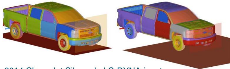
CCSA 2014 Chevrolet Silverado LS-DYNA input run with Radioss (right)
